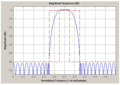
where the passband is from .45 to .55 of normalized frequency, the amount of ripple acceptable in the passband is 1 dB, the first stopband is from 0 to .35 (normalized), the second stopband is from .65 to 1 (normalized), and both stopbands provide 60 dB of attenuation.
